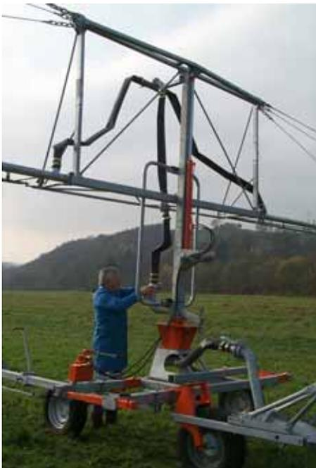
34. For higher crops, the AS 50 can be equipped with a hydraulic high adjustment. With a hydraulic hand pump the boom can be lifted up to a free clearance of 2,5 m. A hose extension is added to the water supply. The two balancing weights are readjusted slightly above ground level.
