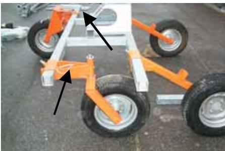
35. Remove locking pin on swivel wheel and loosen it at the wheel (adjustment only for transport with RAINSTAR)
