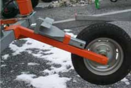
39. During the operation of the AS 50 the draw out hook is uncoupled and fixed in a holding sleeve. The tracking wheel is lowered, the chain engaged and tensioned with the lever. Thereby the tracking wheel is pressed into the ground. With the sliding bolt the tension lever is fixed.
