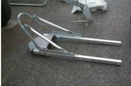
3. Assemble the adjustable shut-off fin according to the plan and connect it up to the horizontal pipe of the Rainstar.
