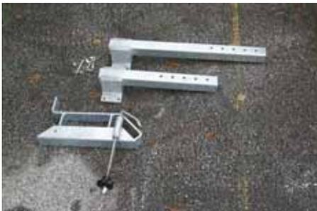
31. Mount the bearing brackets on both side frame members of the Rainstar. The required mounting holes are already available.
