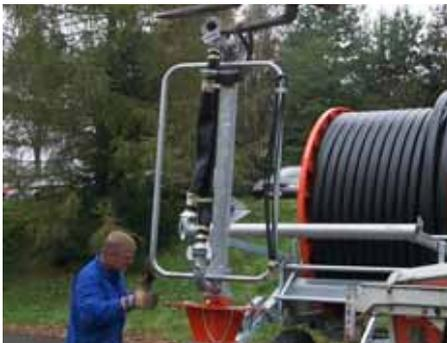
12. Put the center support with the intermediate piece on the flanged plate of the undercarriage and screw it down. Thereby the cart lifting hook points into the direction of the steered front wheel. Depending on the PE-pipe run-in position to the Rainstar, the hose connection is pointing diagonally to the front left or front right.
