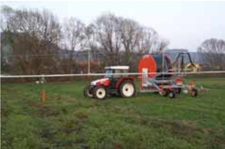
40. When the AS 50 has reached the end position at the Rainstar and the unit has switched off, The Rainstar and the boom can be transported into the next position. First the AS 50 is lifted hydraulically and then it is moved into the next operating position.
