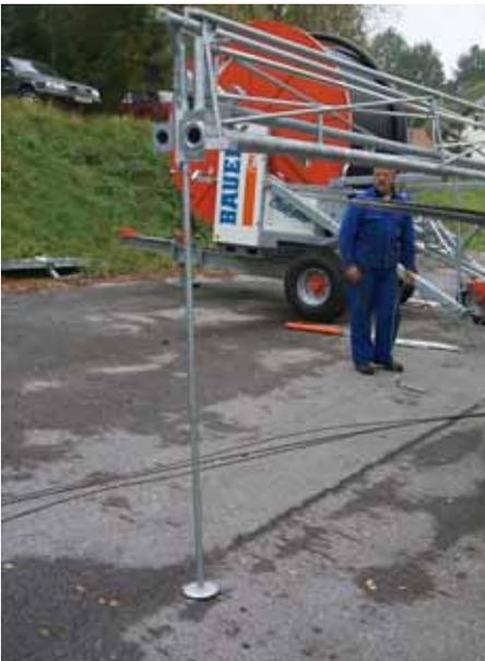
20. Backing up the first boom pipes with the adjustable support avoids swinging of the boom and makes the following assembly easier.
