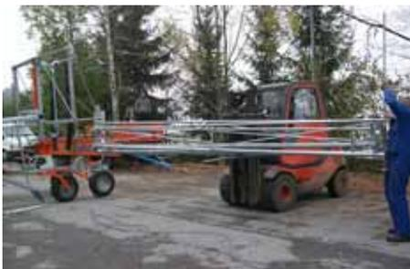
19. The boom pipes must be assembled step by step alternating on the left and on the right and braced with cables. A complete pre-assembled boom package consisting of 4 boom pipes with wind bracing is fixed to the center part with a pin.
