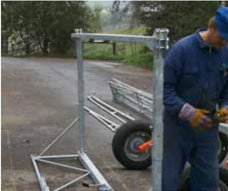
15. Join the upper and lower part of the pendulum center part, add the reinforcement brackets and complete the assembly.
