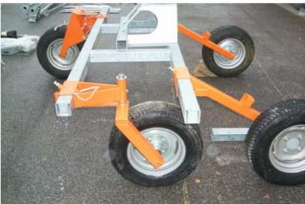
9. Mount the 360° swivelling support wheel on the opposite side. The mounting bracket with the swivel axle points backwards.
