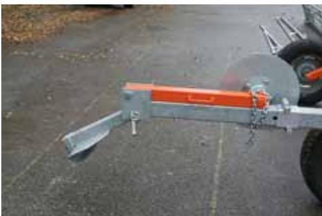
37. Pick up the draw-out hook on the draw bar with the tractor toolbar and pull the boom cart through the field with the boom arms opened up. The pendulum center part has to be locked with the locking bracket during the pull out procedure.
