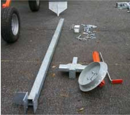
10. Mount the drawbar on the side of the steered wheel, (in line with the PE-pipe). On the 3-wheel cart, the draw bar is mounted in the centre of the cart.
