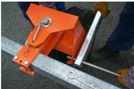
4. The adjustment of the shut-off fin varies depending on the respective Rainstar model. The adjustment has to be made per drawing sent with add on parts in the delivery.
