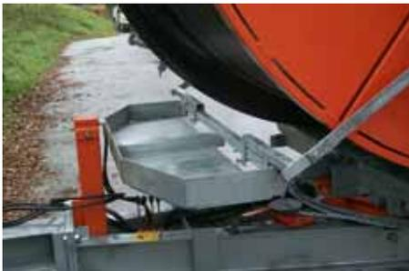
33. Is a Rainstar model E 11 or E 21 used to operate a AS 50, a tray for weight deposit has to be mounted. A weight of about 120 kg (concrete blocks or sand bags) has to be placed in this tray, to ensure sufficient stability of the Rainstar, especially when the boom is lifted on the side of the Rainstar.
