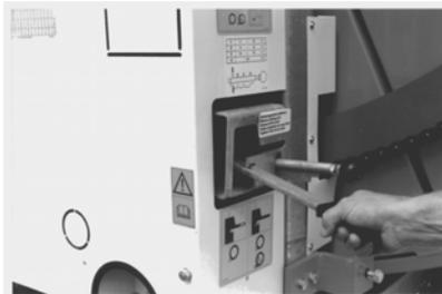
36. Lower hydraulic Rainstar supporting legs and AS 50 slowly. Move gear shift lever to „PE-pipe pull-off“ position. (see Rainstar operating instructions)
