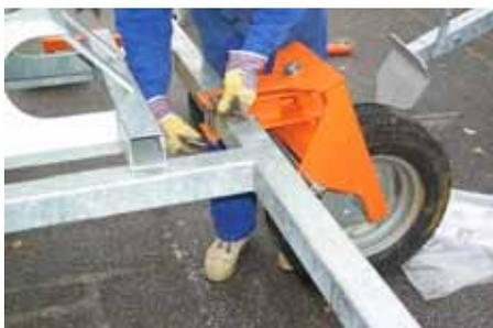
2. Mount the steered front wheel in the middle of the undercarriage.
