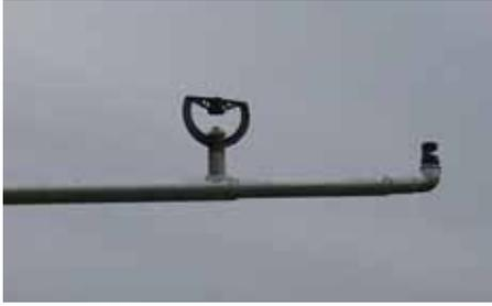
29. Depending on the desired nozzle configuration – turn in spray or rotator nozzles with a teflon tape sealing.
