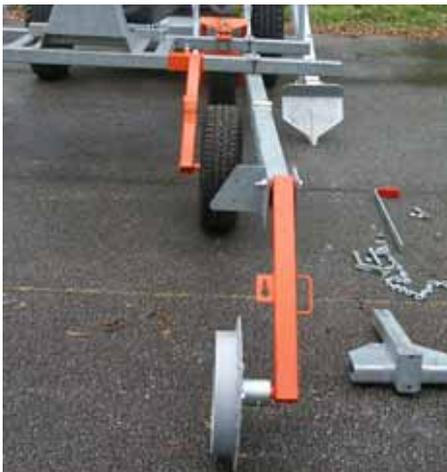
11. Position the tracking wheel support on the drawbar in such a manner that the tracking wheel lies in the tracks of the cart wheels.
